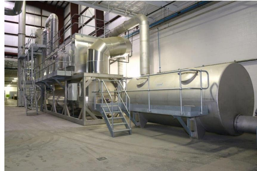
The carrier exhaust air extracts from the shredding, separation and pulverisation stages are introduced through a recuperative heat recovering system where the heat is supplied by the already cleaned air, before going into the catalytic chamber. Heater is used for preheating the process air to achieve the set controlled temperature for the purification process above.
